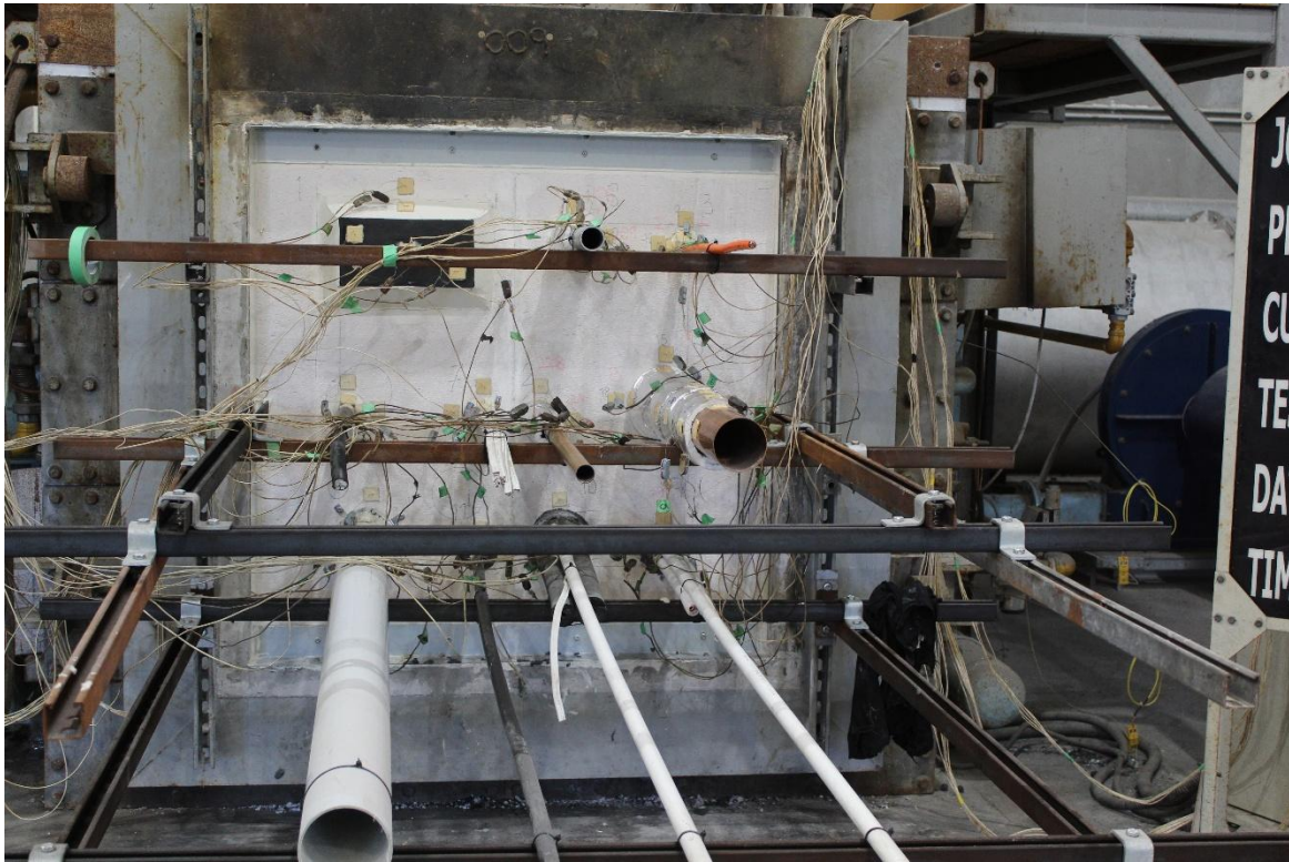
Figure 1 - Unexposed face prior to test commencement
